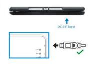
3. To recharge the keyboard, please connect the keyboard to a compatible 5V/0.5A USB charger using a micro-USB charging cable (included). The keyboard is fully functional while it is being recharging.
